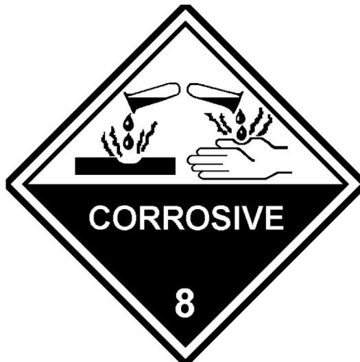
Fig. 3. Corrosive placard. (From Centers for Disease Control, The National Institute for Occupational Safety and Health (NIOSH). Available at http://www.cdc.gov/niosh/ . Accessed July 1, 2014.)
